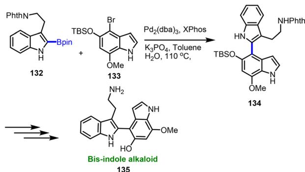
Fig. 25 Total synthesis of a bisindole alkaloid.
