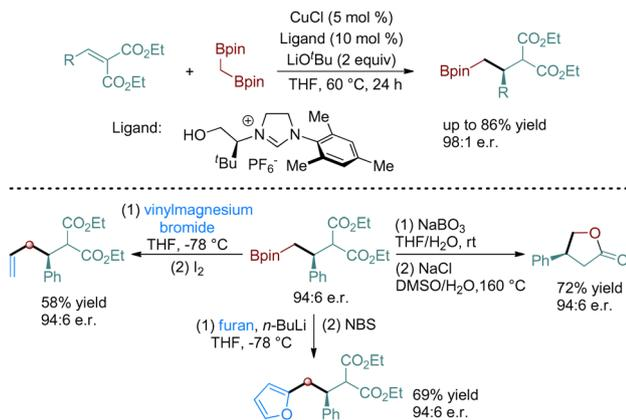
Scheme 24 Cu-catalyzed enantioselective conjugate addition of 1,1-diborylmethane to  $\alpha,\beta$ -unsaturated diethyl diesters.
