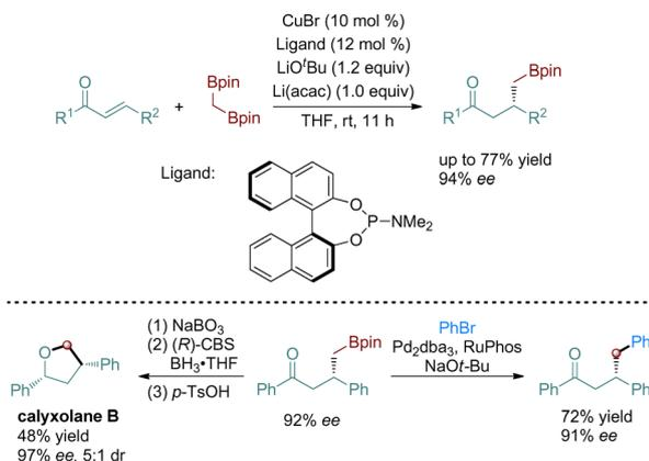
Scheme 25 Cu-catalyzed enantioselective conjugate addition of 1,1-diborylmethane to  $\alpha,\beta$ -unsaturated ketones.
