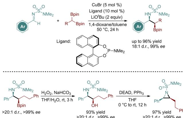
**Scheme 19** Cu-catalyzed enantio- and diastereo-selective 1,2-addition of 1,1-diborylalkanes to *N,N*-dimethylsulfamoylimides.
