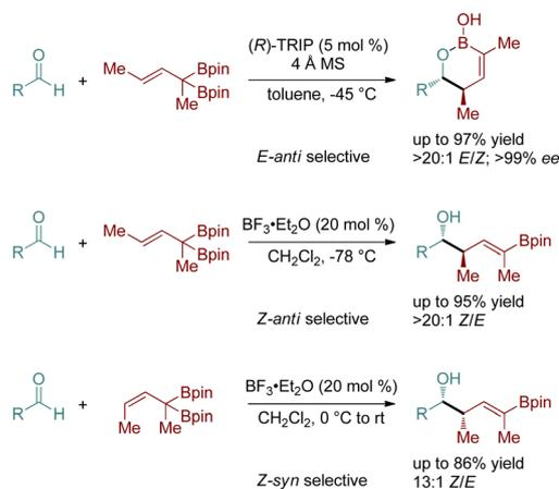
**Scheme 15** Chiral phosphoric acid catalyzed enantio- and diastereoselective 1,2-addition of  $\alpha,\alpha$ -disubstituted *gem*-diboronates to aldehydes.
