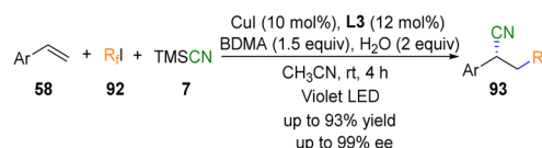
Scheme 27 Photoinduced copper-catalyzed enantioselective cyanofluoroalkylation of alkenes.
