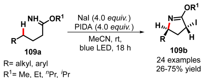
Scheme 109 Nal/PIDA mediated and visible light (blue LED) initiated intramolecular \gamma -C(sp 3 )-H bond amidation (Kumar et al. 147 ).
