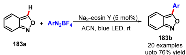
Scheme 183 Eosin Y catalysed C–H arylation of anthranils (Adak et al. 240 ).
