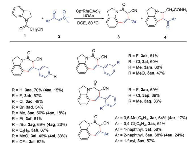
**Scheme 3** Substrate scope of sulfoxonium. Reaction conditions: **1a** (0.2 mmol), **2** (0.3 mmol), Cp\*Rh(OAc)<sub>2</sub>·H<sub>2</sub>O (8 mol%), LiOAc (25 mol%), *t*-AmOH (2 mL), 80 °C, 12 h, isolated yield.
