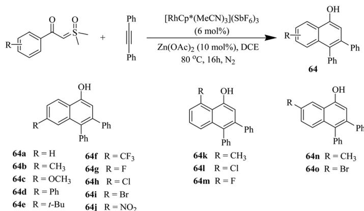
Scheme 74 Redox neutral annulation of sulfoxonium ylides with alkynes.
