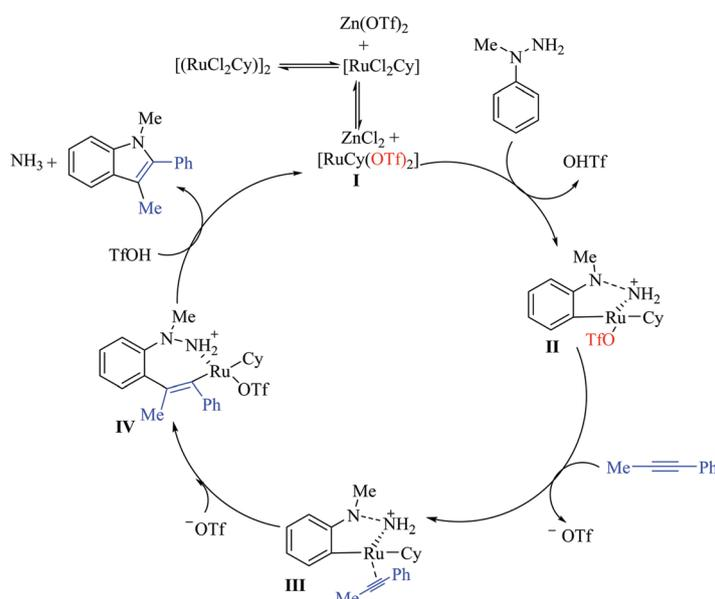
Scheme 63 Mechanism for the synthesis of indoles from *N*-hydrazines.
