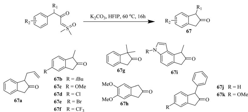
Scheme 78 Intramolecular cyclisation of  $\alpha$ -carbonyl sulfoxonium ylides.
