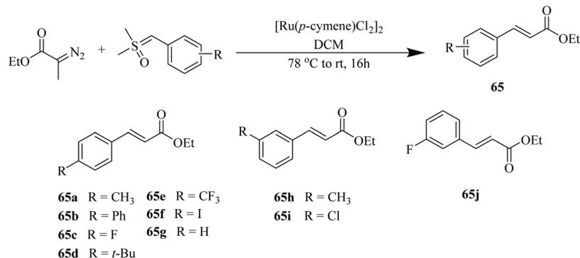
**Scheme 76** Ru-Catalyzed cross olefination between carbene precursor sulfoxonium ylide and diazo compounds.
