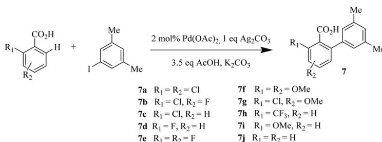
Scheme 8 Synthesis of 2-aryl-6-substituted benzoic acids by switching off the decarboxylation process.
