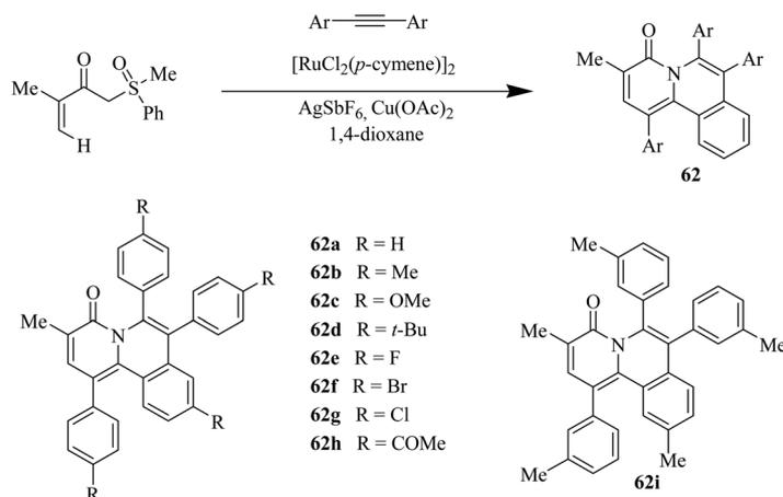
Scheme 72 Ru-Catalyzed synthesis of pyrido-fused isoquinolines.
