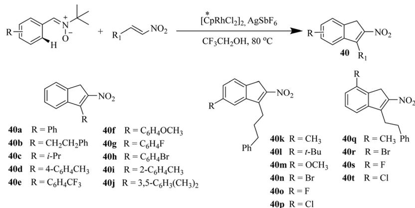
Scheme 48 Rh(III) catalyzed synthesis of nitro-functionalized indenes.
