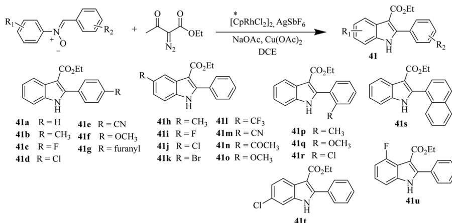
Scheme 49 Rh(III) catalyzed synthesis of 2,3-disubstituted NH indoles.
