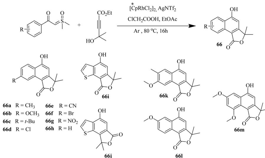
Scheme 77 Synthesis of furanone fused 1-naphthols by using a domino reaction.
