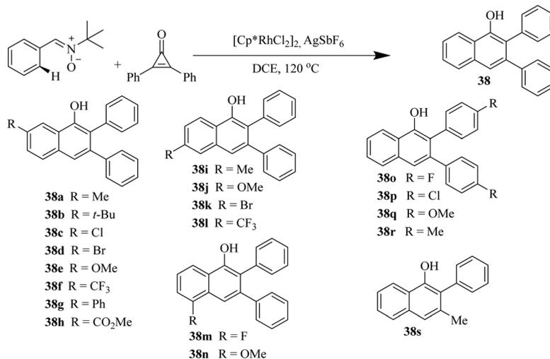
Scheme 45 Rh catalyzed coupling reaction with cyclopropanones.
