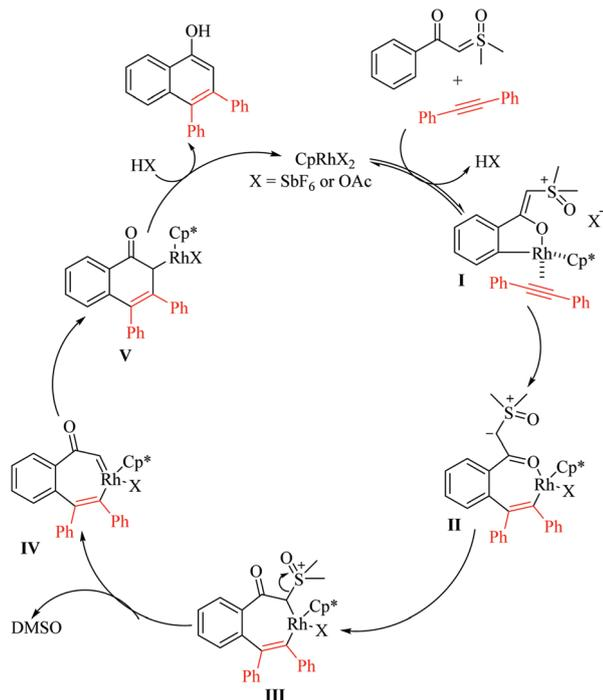
**Scheme 75** Mechanism for redox neutral annulation of sulfoxonium ylides with alkynes.
