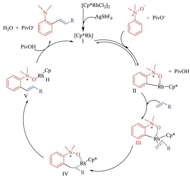
Scheme 40 Mechanism for the synthesis of *ortho*-substituted olefinated derivatives of tertiary amines.
