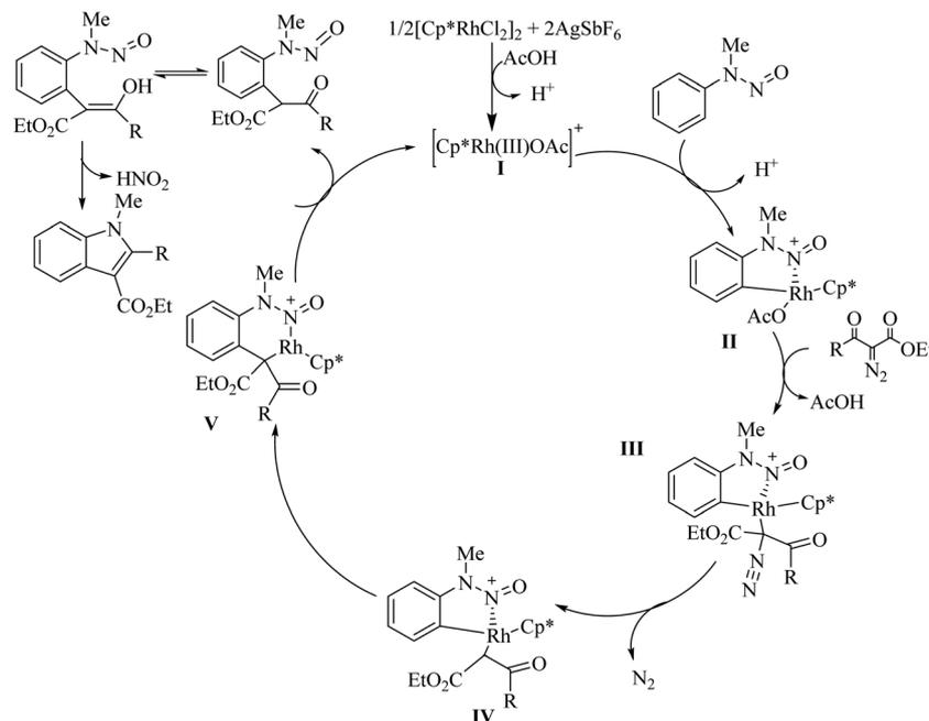
Scheme 54 Mechanism for Rh-catalyzed synthesis of indoles.
