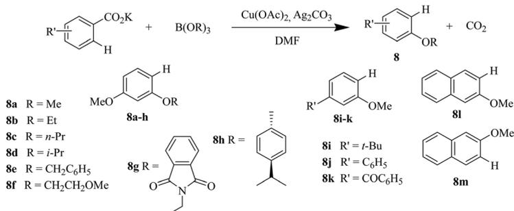
Scheme 9 Synthesis of aryl ethers from benzoates with the protodecarboxylation process.
