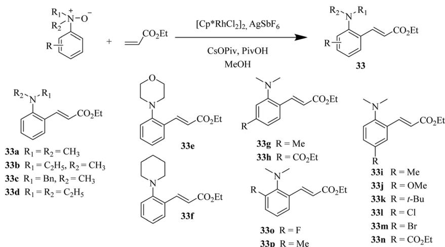
Scheme 39 Synthesis of *ortho*-substituted olefinated derivatives of tertiary amines.
