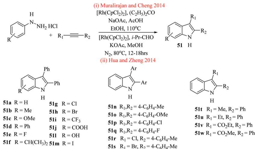
Scheme 60 Rh(III) catalyzed hydrazine directed redox neutral synthesis of indoles.
