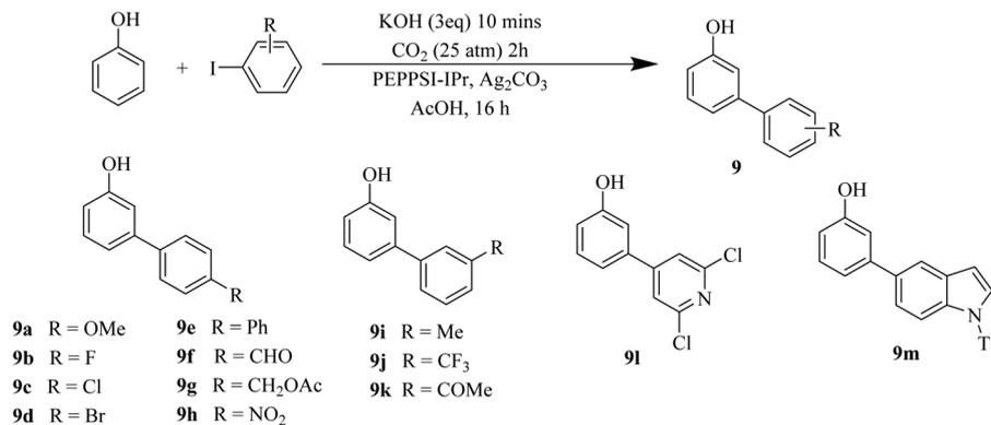
Scheme 10 Synthesis of *meta*-substituted phenols.
