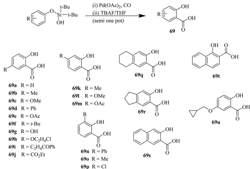
Scheme 80 Pd(II)-Catalyzed synthesis of salicylic acids from phenols.
