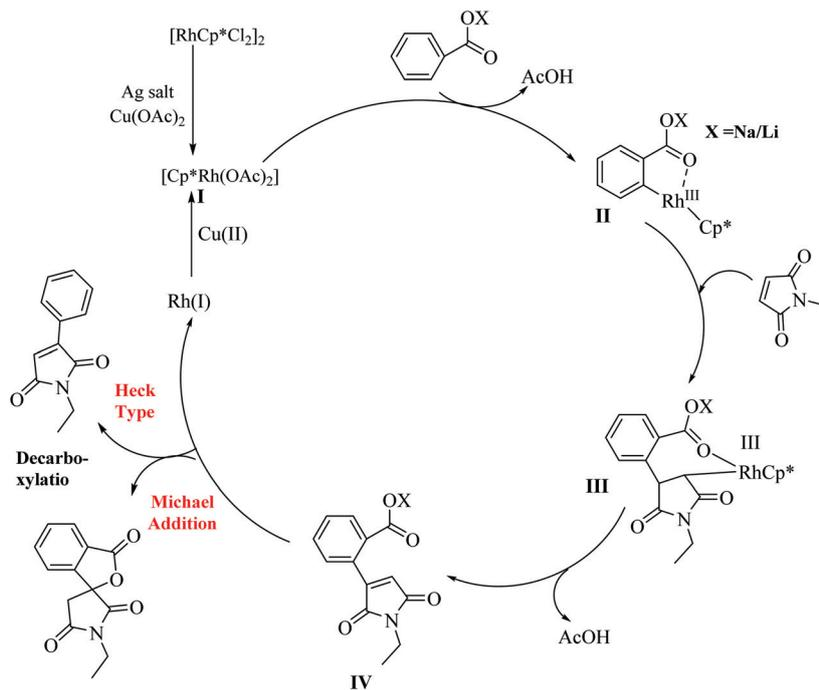
Scheme 32 Plausible mechanism for the switchable decarboxylative rhodium(III) catalyzed Heck type and [4+1] annulation reactions with maleimides.
