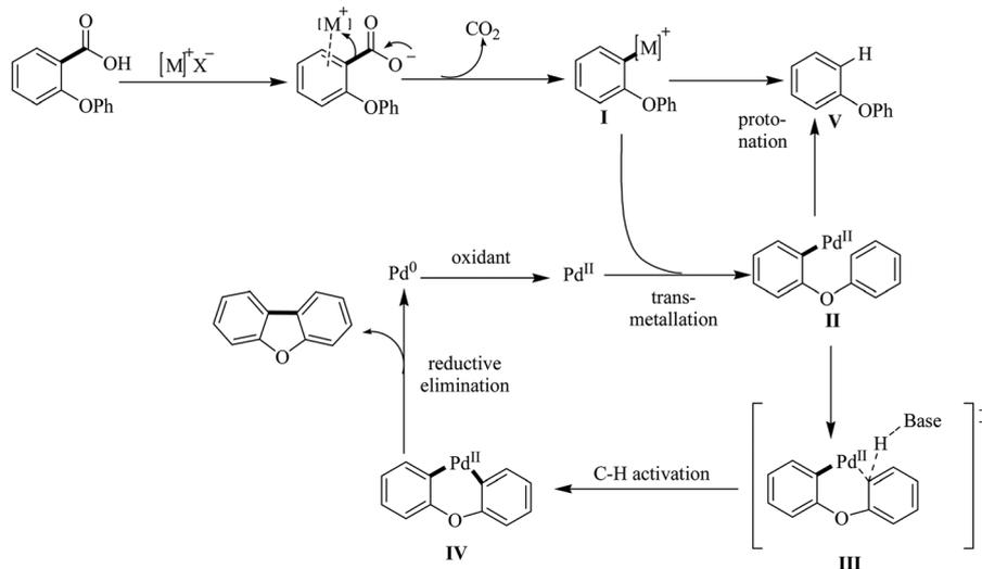
Scheme 3 Plausible reaction mechanism for intramolecular arylation of 2-phenoxybenzoic acids.
