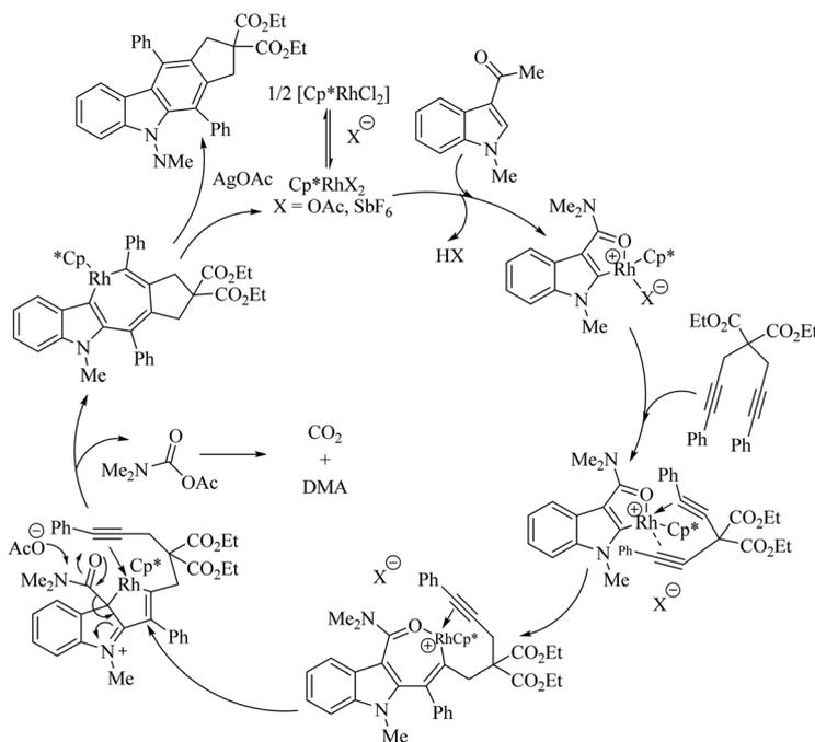
Scheme 70 Mechanism for the cascade reaction between amide substituted indoles and diynes.
