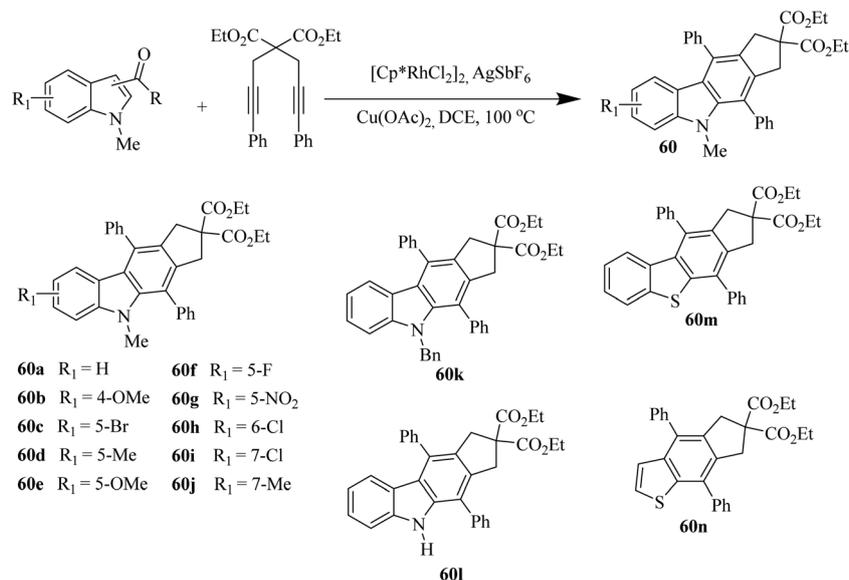
Scheme 69 Rh(III) catalyzed cascade reaction between amide substituted indoles and diynes.
