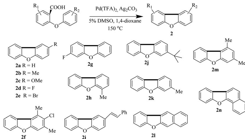
Scheme 2 Intramolecular arylation of 2-phenoxy benzoic acid for dibenzofuran formation.
