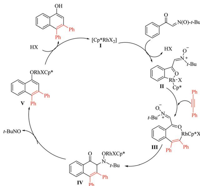
Scheme 47 Mechanism for redox neutral synthesis of naphthols.
