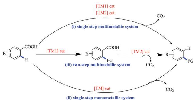
Fig. 2 Three methods of transition metal catalyzed C–H functionalization directed by carboxylic acids.
