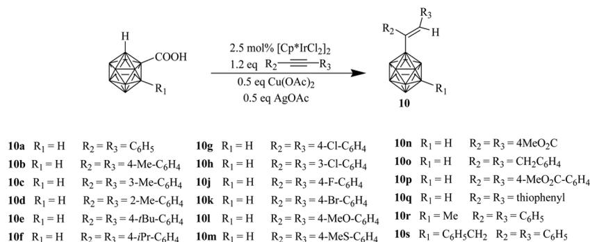
Scheme 11 Synthesis of a series of B-(4)-alkenylated-*o*-carboranes.
