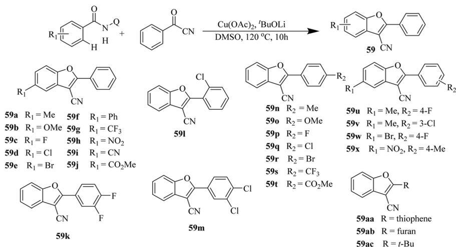
Scheme 68 Synthesis of 2,3-disubstituted benzofurans from benzamides and benzoylacetonitriles.
