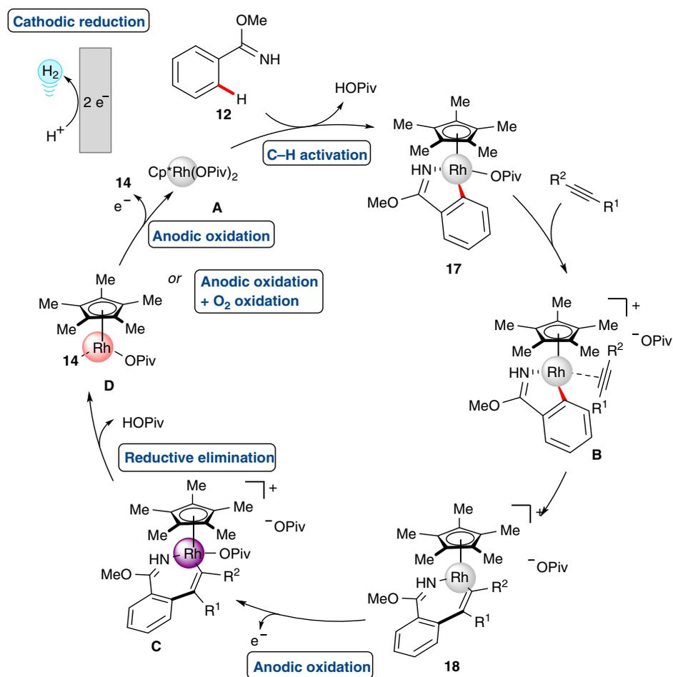
**Scheme 10** | Proposed catalytic cycle for flow-rhoda-electro-catalyzed alkyne annulation.
