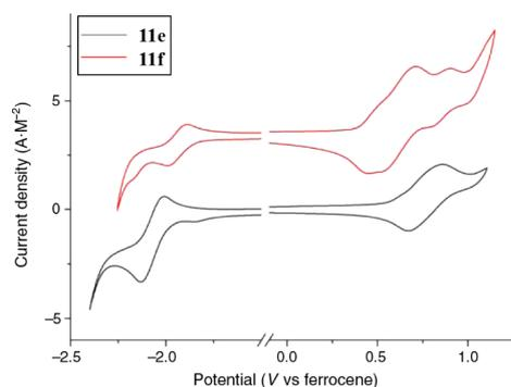
**Scheme 7** | (a) Photoabsorption and (b) CV of **11e** and **11f**.
