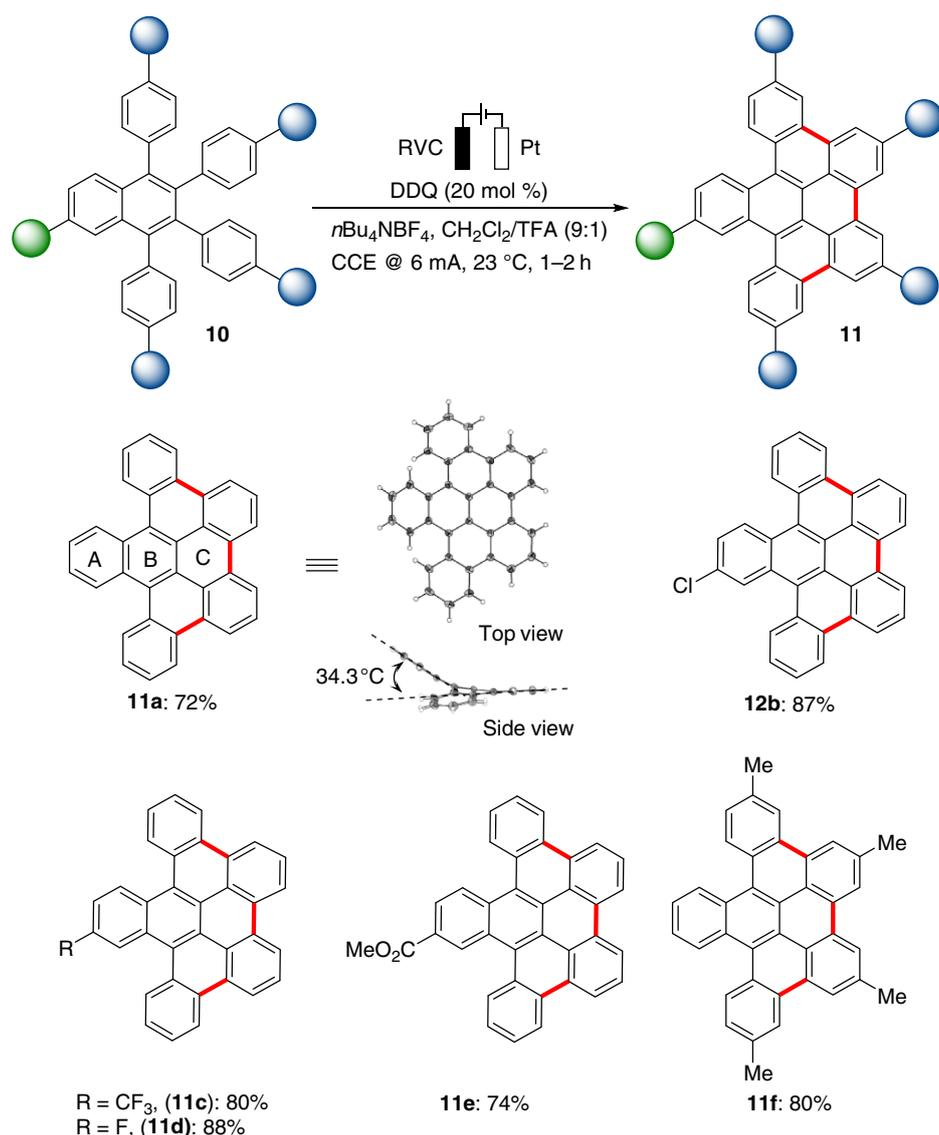
**Scheme 6** | Late-stage diversification by DDQ-catalyzed electrochemical cyclodehydrogenation.
