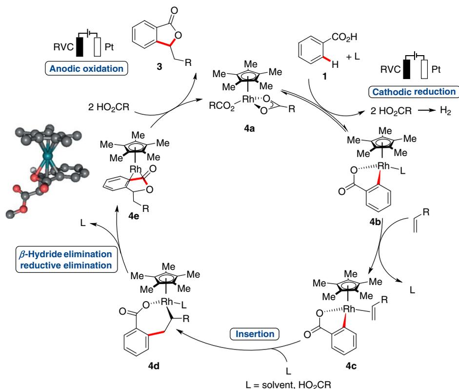
**Scheme 3** | Plausible catalytic cycle for alkenylation.
