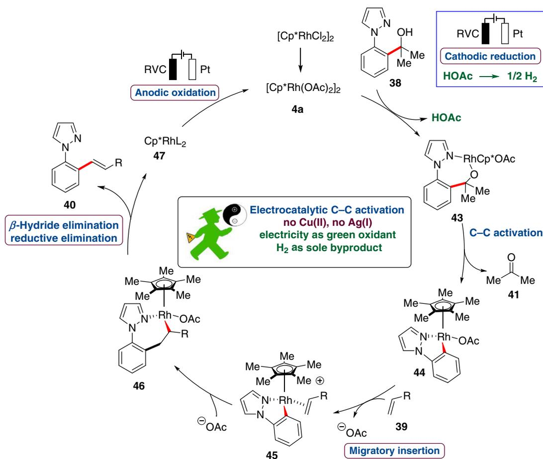
**Scheme 19** | Plausible catalytic cycle of rhodaelectro-catalyzed C–C alkenylation.
