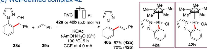
**Scheme 18** | (a–e) Key mechanistic findings of rhodaelectro-catalyzed C–C alkenylation.
