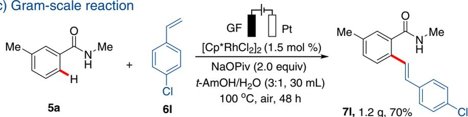
**Scheme 4** | (a–c) Rhodaelectro-catalyzed C–H alkenylation and gram-scale reaction.
