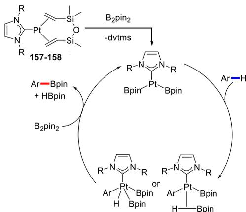
It was proposed that the coordinatively unsaturated Pt–NHC complex reacts with B<sub>2</sub>pin<sub>2</sub> to give [Pt(NHC)(Bpin)<sub>2</sub>], followed by C(sp<sup>2</sup>)–H activation via  $\sigma$ -bond metathesis or oxidative addition to give Pt(IV).
