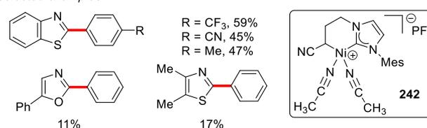
C-H arylation. The authors proposed that the Ni(II)-NHC precatalyst is activated by the dimerization of benzothiazole. In 2018, Ong and co-workers reported Ni(cod)<sub>2</sub>/IPr-catalyzed direct C(sp<sup>2</sup>)-H arylation of azoles with anisoles by a dual C-H/C-O activation pathway (Scheme 201).<sup>376</sup> The reaction requires stoichiometric amounts of a Grignard reagent, and the
