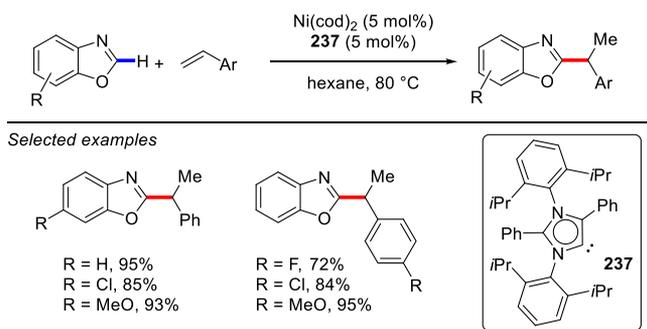
heteroarene bond to give the [Ni(NHC)(H)(Ar)] intermediate, olefin insertion, and reductive elimination. The C–H activation step is likely facilitated by the more flexible steric environment of the abnormal NHC ligand.
