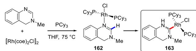
Currently, the major applications of Rh–NHC complexes in C–H activation include the following processes: (1) pyridine-directed C(sp<sup>2</sup>)–H arylation and alkylation; (2) C(sp<sup>2</sup>)–H borylation; (3) 2-fold C–H activation via Rh–NHC intermediates; (4) C(sp<sup>3</sup>)–H functionalization; and (5) C–H/C–D exchange.
