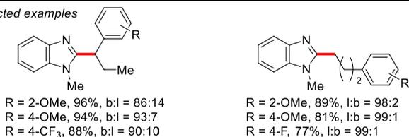
Now, they found that the standard monometallic Ni–NHC catalysis protocol (Ni(cod)<sub>2</sub>/IMes, toluene, 100 °C) leads to the formation of branched C2–H functionalization products by alkene isomerization, while bimetallic Ni–Al catalysis (Ni(cod)<sub>2</sub>/IPr/AlMe<sub>3</sub>, toluene, 100 °C) affords linear C2–H functionalization adducts through steric control of the olefin insertion.
