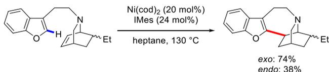
In 2015, Montgomery and co-workers identified the IMes-based Ni-NHC complex **241** as a highly active catalyst for the C(sp<sup>2</sup>)-H alkenylation of acidic C-H bonds in arenes and heteroarenes (Scheme 197).<sup>372</sup> Remarkably, they found that
