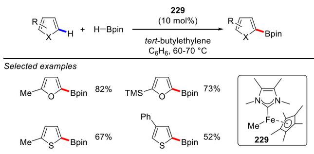
occurred regioselectively at the C2 or C5 positions of the furan and thiophene ring and showed relatively broad substrate scope. Mechanistically, C-H activation occurs at the Fe-NHC complex **229** with a concomitant loss of methane. The reaction with pinacolborane generates the final product.
