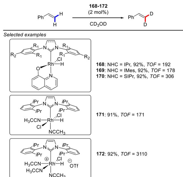
deuteration reaction most efficiently, consistent with a more facile olefin coordination and insertion in this complex. On the other hand, removal of the chloride ligand led to catalytically inactive complexes.
