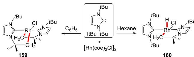
that this Rh(I) complex undergoes a solvent-dependent intramolecular C(sp<sup>3</sup>)–H bond activation process to give **159** through double C(sp<sup>3</sup>)–H activation in benzene or **160** through mono C(sp<sup>3</sup>)–H activation in hexane, respectively.
