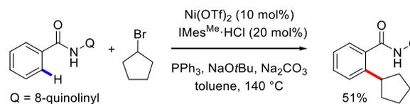
alkylation with challenging secondary alkyl halides directed by the 8-aminoquinolinyl group is facilitated by using a catalyst system based on Ni(OTf)<sub>2</sub>/IMes<sup>Me</sup> and PPh<sub>3</sub> (Scheme 199).<sup>374</sup> The use of an NHC ligand is critical for the success of this reaction.
