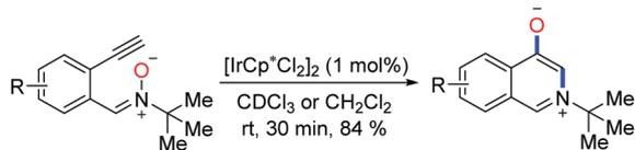
Scheme 2  $[\text{IrCp}^*\text{Cl}_2]_2$ -catalysed intramolecular O-atom transfer.
