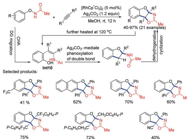
**Scheme 10** Rh(III)-Catalysed cascaded C–H activation/acetamido migration/dioxygenation for the preparation of dihydrobenzofuro[2,3-*d*]oxazole skeleton.
