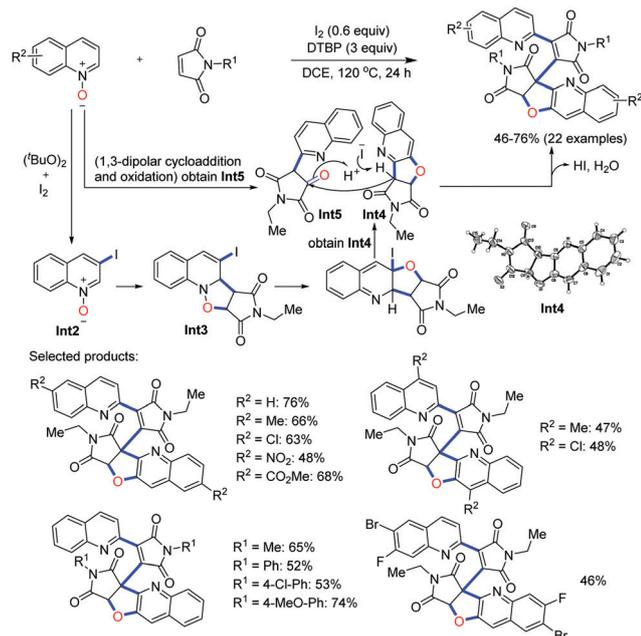
Scheme 4  $\text{I}_2$ -Mediated tandem iodization/[3+2]cycloaddition/nucleophilic addition for the synthesis of polyheterocycles.
