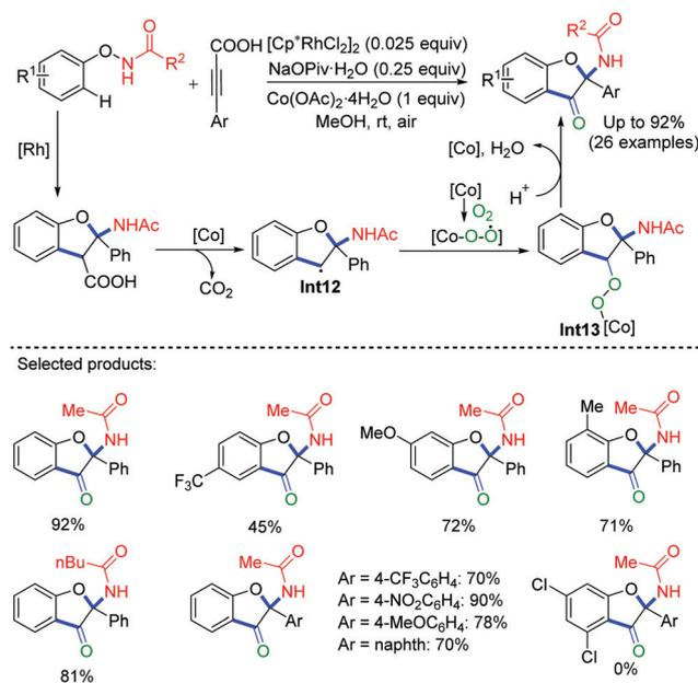
**Scheme 13** Rh(III)-Catalysed cascaded C–H activation/acetamido migration and [Co]-mediated decarboxylation/radical coupling for the preparation of benzofuran-3(2*H*)-ones.
