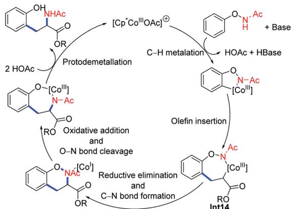
**Scheme 15** Proposed catalytic cycle for C–H activation with subsequent acetamido migration.
