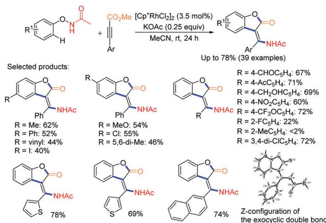
**Scheme 12** Rh(III)-Catalysed cascaded C–H activation/acetamido migration/isomerization/lactonization for the preparation of benzofuran-2(3*H*)-ones.
