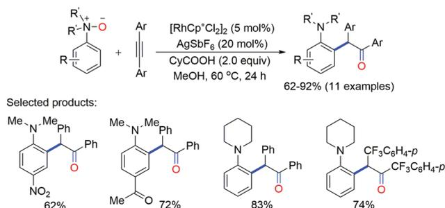
Scheme 7 Rh(III)-Catalysed tandem C–H activation/oxygen atom transfer using tertiary aniline *N*-oxides as the substrate.
