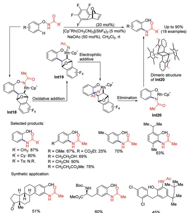
**Scheme 18** Rh(III)/bicyclic olefin co-catalysed intramolecular *ortho*-C-H amidation for the synthesis of *O*-amidophenol.
