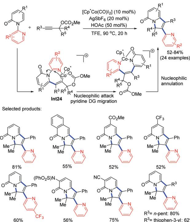
Scheme 24 Co(III)-Catalysed cascaded C–H activation/pyridyl migration/cyclization for the synthesis of indolizinone scaffolds.
