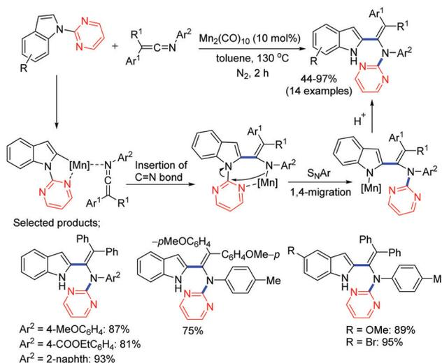
Scheme 22 Mn(I)-Catalysed C–H alkenylation/pyrimidinyl migration for the preparation of 2-enaminylated indoles.
