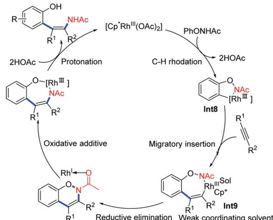
**Scheme 9** Proposed catalytic cycle for C–H activation with acetamido migration.
