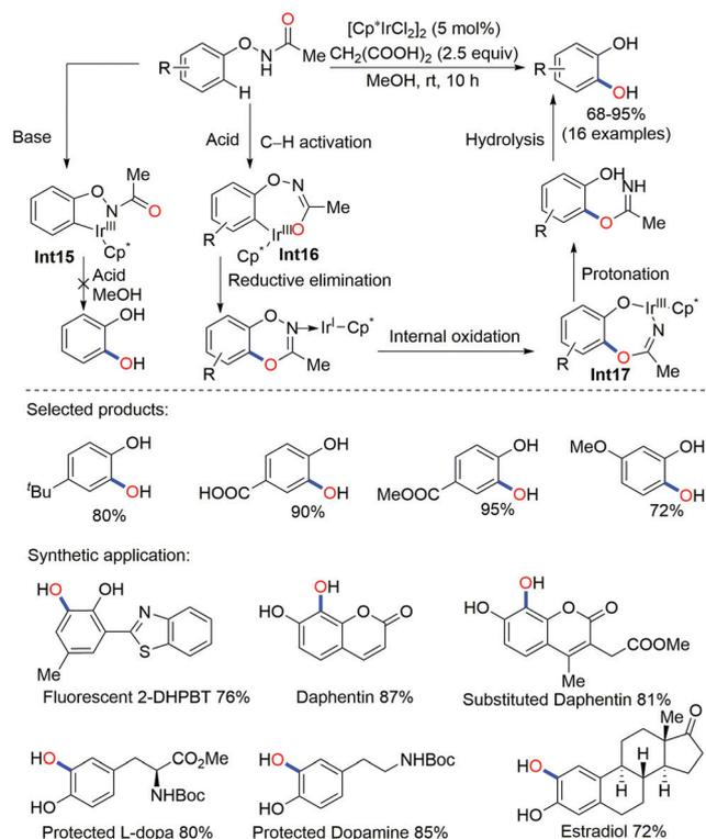
**Scheme 17** Ir(III)-Catalysed cascaded intramolecular C-H activation/OTA for the synthesis of catechols.
