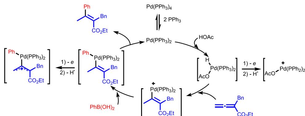
same period, the group of Oh reported a quite similar catalytic system using 3% of  $\text{Pd}(\text{PPh}_3)_4$ , in the presence of 10% of acetic acid applied to mono- and disubstituted allenenes.<sup>124</sup>
