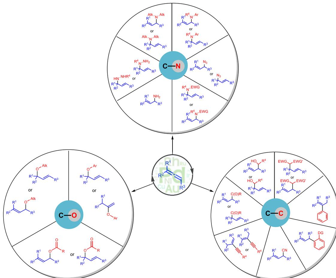
**Figure 4.** Metal-catalyzed intermolecular hydrofunctionalization of allenes.
