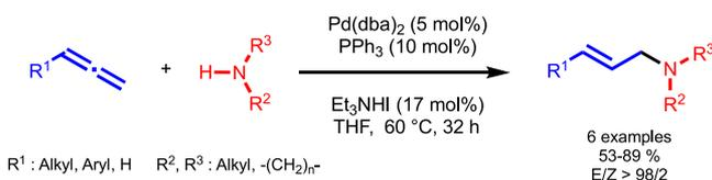
A few years later, in 1997, Yamamoto and co-workers described a related method involving the formation of a hypopalladium(II) intermediate by oxidative addition of acetic acid to a Pd(0) complex.<sup>25</sup> With this catalyst in hand they performed the hydroamination of monosubstituted allenes with various amines such as diethyl iminoacetate or tosylamine.
