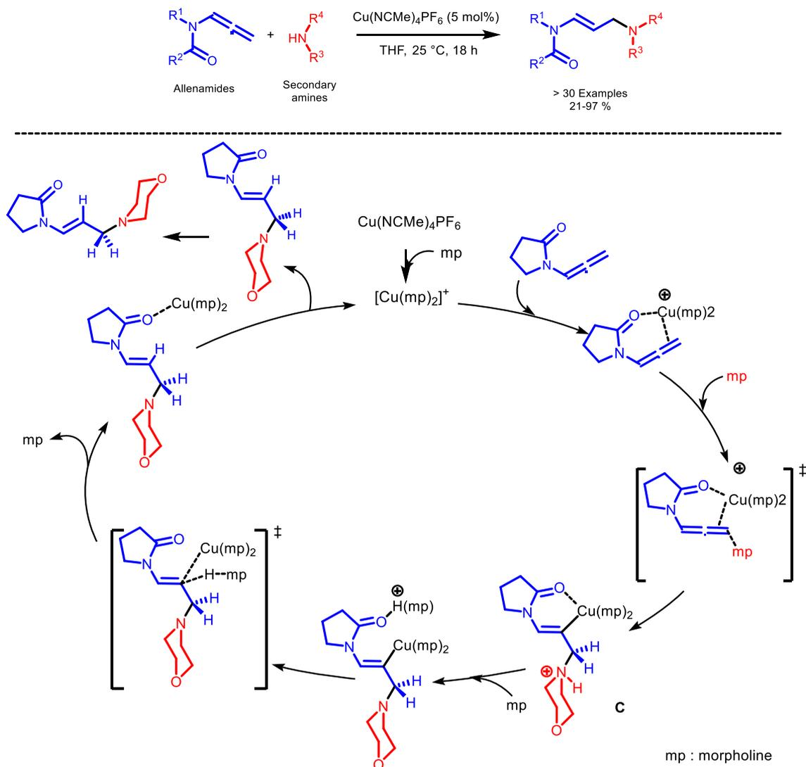
Scheme 11. Cu-Catalyzed Hydroamination of *N*-Allenylazoles and *N*-Allenylsulfonamides with Secondary Amines
