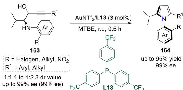
Scheme 48. Synthesis of axially chiral arylpyrroles via chirality conversion strategy.<sup>[82]</sup>
