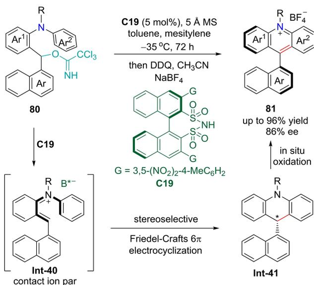
**Scheme 27.** Synthesis of atropisomeric acridinium salts via asymmetric intramolecular cyclization reaction.<sup>[49a]</sup>
