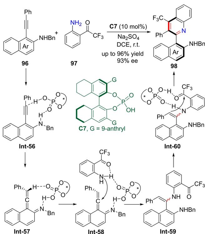
**Scheme 32.** Asymmetric heteroannulation of alkynes to construct axially chiral isoquinoline-naphthylamine skeletons.<sup>[55]</sup>
