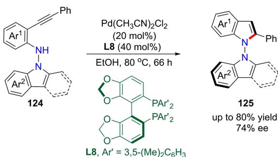
**Scheme 39.** Atroposelective synthesis of N–N bisindole via Pd-catalyzed intramolecular reaction.<sup>[66]</sup>
