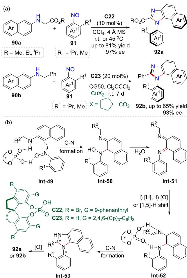
**Scheme 30.** Synthesis of axially chiral *N*-arylbenzimidazoles of naphthylamine derivatives and nitrosobenzene.<sup>[53]</sup>
