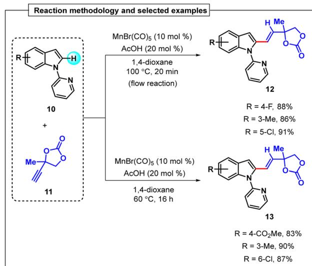
Scheme 9 Synergistic manganese(I) C–H activation catalysis in continuous flow.
